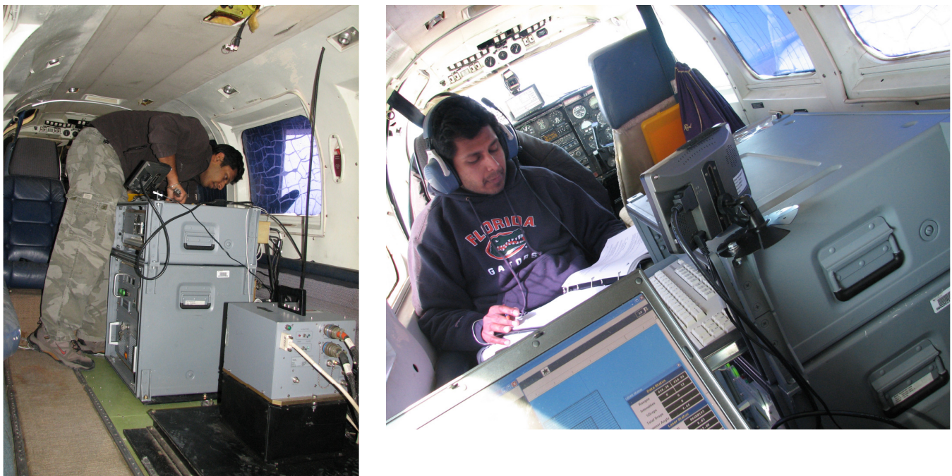
Figure 1 – NCALM Gemini ALTM and waveform digitizer installed in a Piper PA-31.
